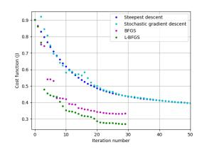
Steepest Descent: For a control vector  $X_i$  and gradient  $g_i$ , let  $X_{i+1} = X_i - ag_i$  using some learning rate a
