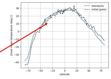
Set up as an optimization problem: minimize  $J = (\Sigma (T_i - T_{i,Target})^2)^{0.5}/N$
